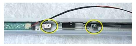
10. Tilt up the antenna receptor to remove it from the left side of the bezel assembly.
