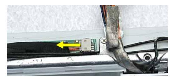
6. Remove the reed switch cable assembly.
