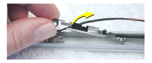
11. Unwrap the tape that secures the AirPort Card antenna to the cable bundle.
