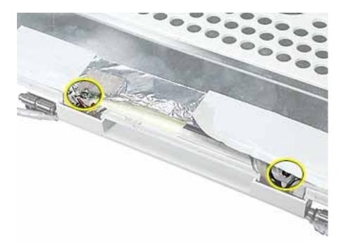
6. Tilt up the display assembly and pull straight down on the display clutch cover.
