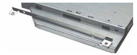
14. Install the replacement optical drive, and reassemble and test the computer.
