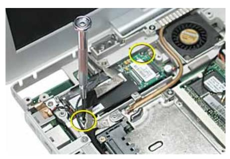
3. Without straining the LVDS cable, peel off the clear tape.
