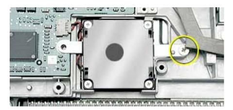
2. Lift the fan and bracket from the computer, and disconnect the connector from the logic board. (Use a black stick, if necessary.)
