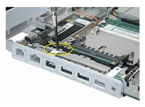
2. Tilt down the I/O bezel and remove it from the computer frame.
