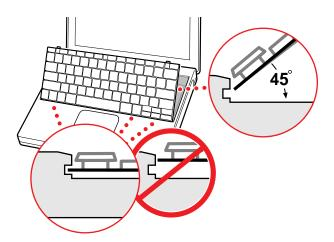
• Pull down on the keyboard release tabs and then press down on the top portion of the keyboard to secure it in place.
