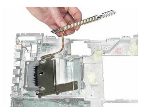
7. Turn over the heat spreader and notice the placement of the thermal pad on the other side. If replacing the heat spreader, make sure it has the thermal pad.
